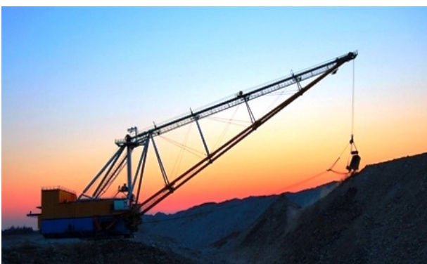
Dragline used in open cast mining.
