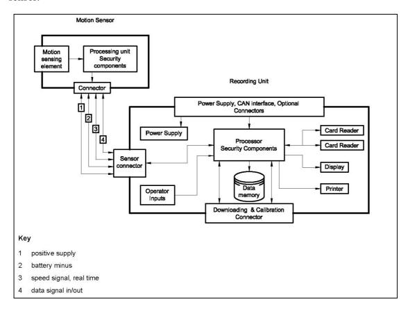
Figure 1: Schemata of typical digital recording equipment
