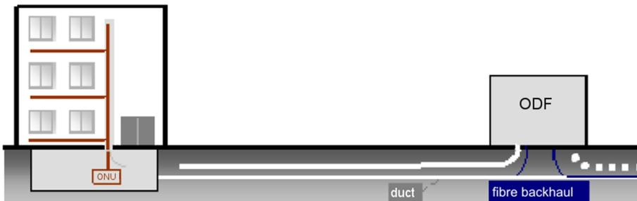
**FTTC/VDSL** – Fibre to the cabinet: a significant part of network is still built with copper but enables operators to provide enhanced speeds on the basis of different technologies, such as [vectoring](#) and [G.Fast](#).
