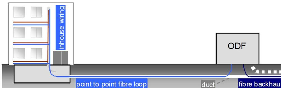
**FTTB** – Fibre to the building: the final link to the end-users' premises is still built with copper.
