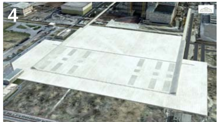
For worker protection a 90,000 square metre concrete work area will be laid
