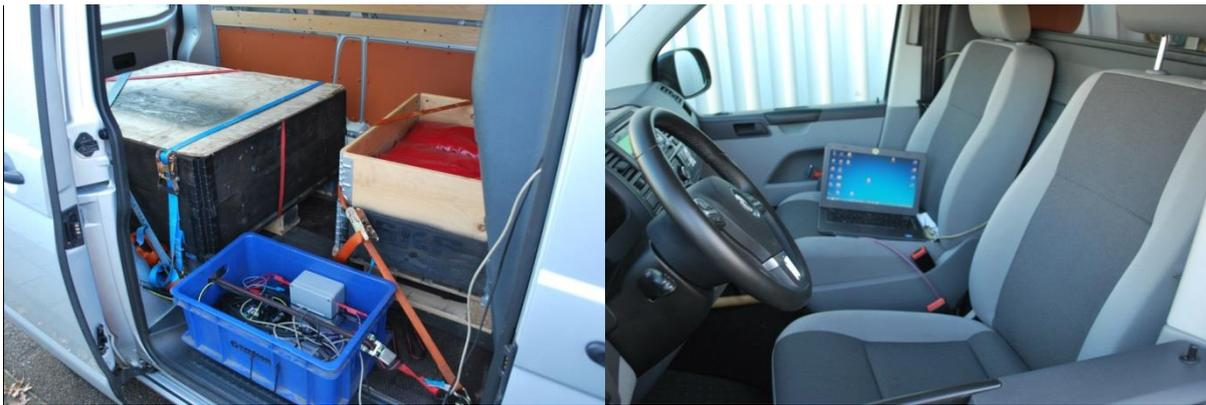
Figure 9: Left: Load packages (black box) and data logger of the SEMS (blue cradle) used in on-road testing of a light commercial vehicle.
