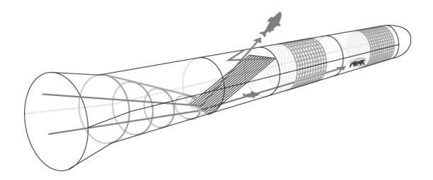
Schematic illustration of a size and species selective trawl. Entering fish are led towards the trawl floor and grid via a leading funnel. Larger fish are then led out of the trawl by the grid while smaller fish and Norway lobster pass through the grid and enter the codend. The full square mesh codend enhances escapement of small fish and undersized Norway lobster. The square mesh codend shown in the diagram is required only in Skagerrak and Kattegat.
