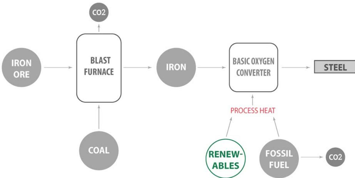
Inside the blast furnace, carbon particles initially react with a limited amount of oxygen to produce carbon-monoxide. This carbon monoxide gas will then chemically react with the iron oxide particles, producing iron and CO<sub>2</sub>.
