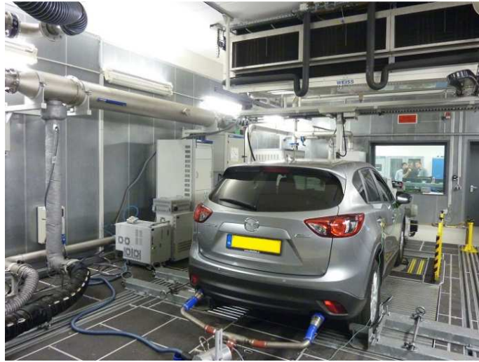
Figure 2 A vehicle tested in the laboratory on a two-wheel chassis dynamometer (roller bench)
